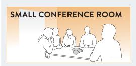
Place the Konftel 300/300IP/300IPx in the middle of the table. The microphones pick-up area is up to  $30 \text{ m}^2/300 \text{ sq ft.}$
